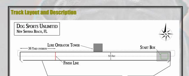
The above diagram displays the dimensions and layout of the Fast CAT track at the Dog Sports Unlimited New Smyrna Beach facility. The course is located on the northern most section of the property and is oriented in an east-west direction. The timed portion of the track is the 100 yards. There is 36 yards of track beyond the finish line.
